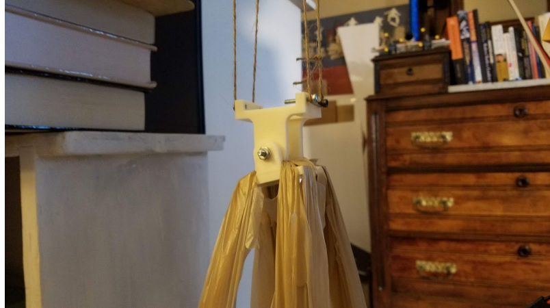
Load testing the forward motor pivot mount. A couple weights are suspended in the bags, simulating the thrust of the motor in the forward direction.
